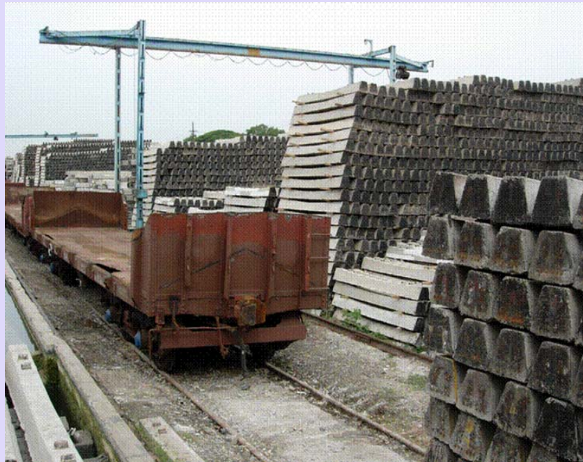
(n) Storage and dispatching of sleepers
