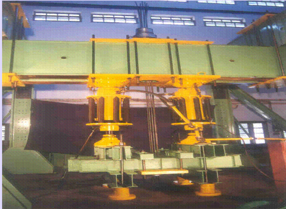
Figure 1-4.11 Testing of an anchorage device
