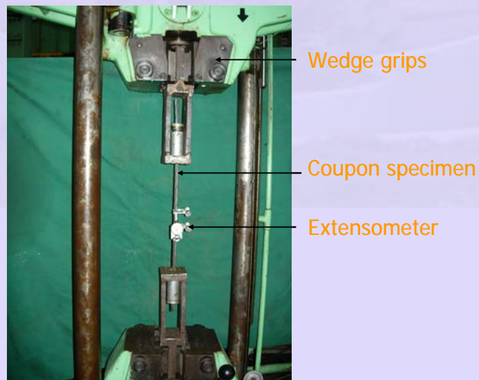
(a) Test set-up
