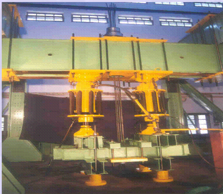
Figure 1-7.11 Set-up for fatigue testing of strands
