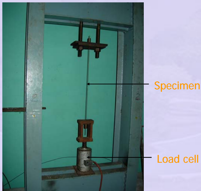
(a) Test of a single wire strand
