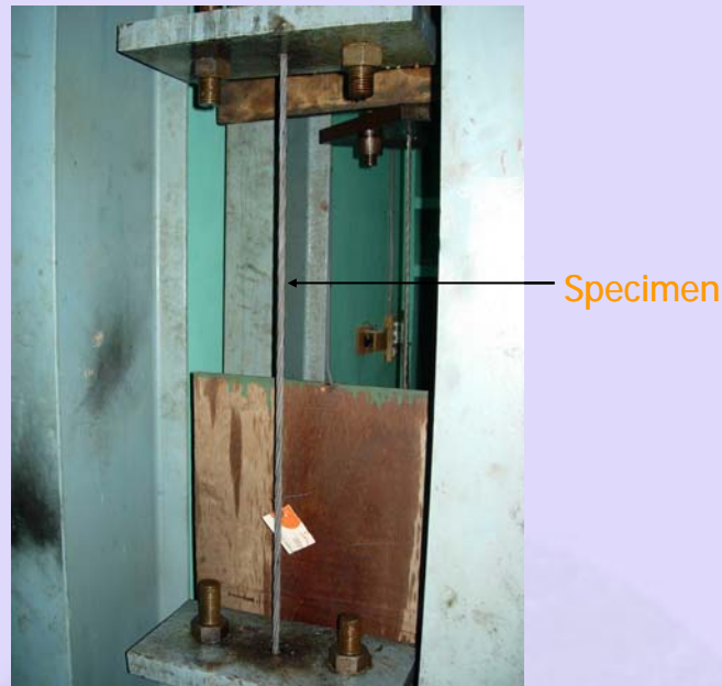
(b) Test of a seven-wire strand
