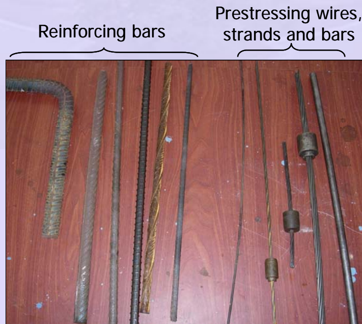
Figure 1-7.2 Forms of reinforcing and prestressing steel
